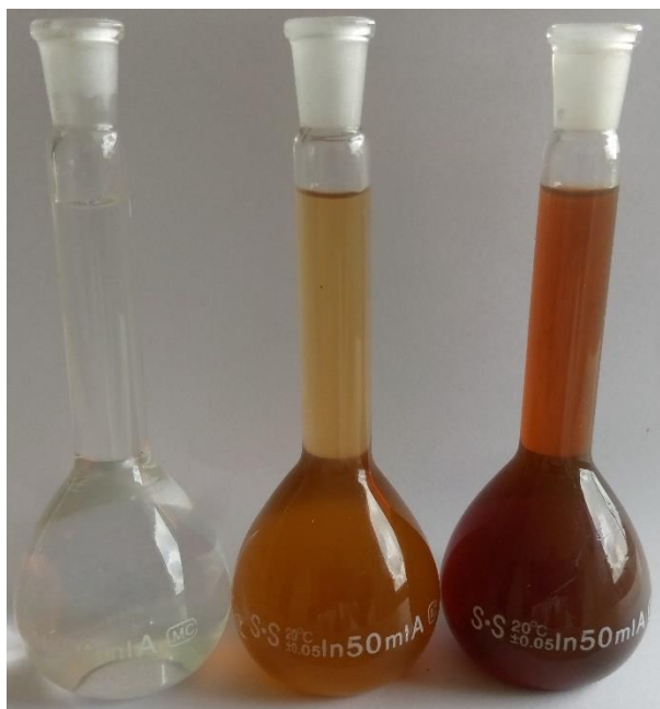
Fig.1 Change of colour during the synthesis: left silver nitrate, middle Ocimum basilicum leaf extract, right silver nanoparticles
