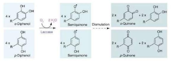
Figure. 1. Oxidation of flavonoids with Laccase
